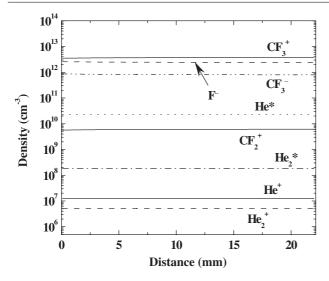
**Figure 4.** The predicted densities of the ions and excited helium species in the  $CF_4$  and He atmospheric-pressure plasma.
