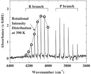
**Figure 2.** Infrared absorption spectrum of HF taken during the titration of F atoms with  $H_2$  in the CF<sub>4</sub>–He plasma afterglow.
