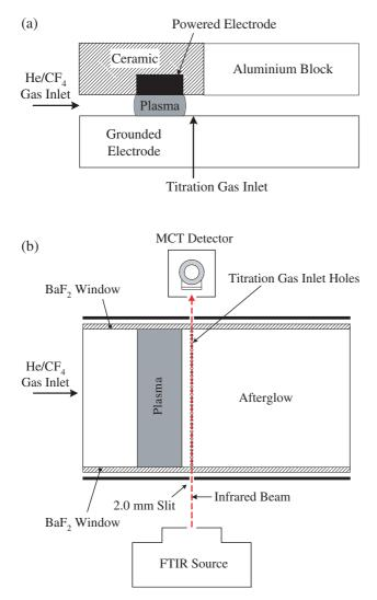
**Figure 1.** (*a*) Side view of the plasma source. (*b*) Top view of the interior of the plasma source.
