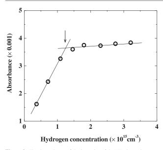
**Figure 3.** The dependence of the intensity of the HF absorption peak at  $4039.7 \text{ cm}^{-1}$  on the H<sub>2</sub> concentration in the plasma afterglow. The arrow denotes the titration point.
